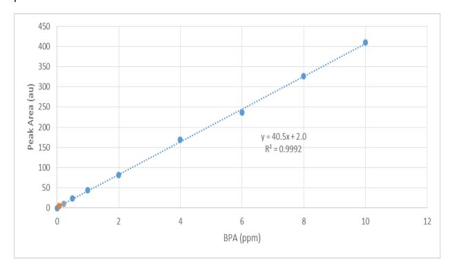
This curve calibrates, or gives us a baseline of behavior for this particular chemical, BPA; and allows of to quantify our results. The R squared value of the trendline equation is 0.9992, the limit of detection occurs at 0.07289 ppm, and the limit of quantification occurs at 0.22088 ppm. This indicates a fairly sensitive test to both detect and be able to quantify the amount of BPA in the following samples.
