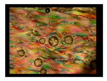
This is a picture of one of the more well-behaved samples between polarizers. The circles are 5CB droplets. The blurs of rainbow light are domains of aligned DSCG liquid crystal molecules, dissolved in water.
