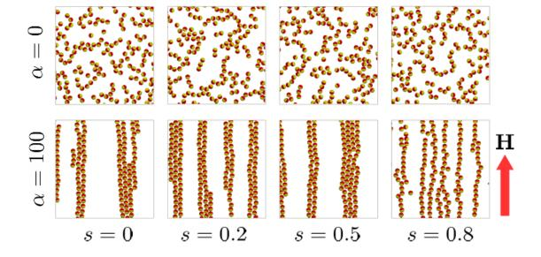
In these snapshots it can be seen how the particles aggregation is enhanced by the application of an external magnetic field and how the shift ratios affect this process as it increases. This happens because the particles have now (at high shift ratios) more unstable bonds with each other and the proximity of other particles to an already formed chain will just increment the energy of the bond and therefore, be repelled as it doesn't lead to a lower and stable energy state.
